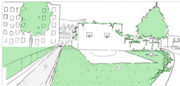
A Permeable gravel path. B Opportunities to make impermeable surfaces permeable. Opportunities for creating of lawn and tree planting C Potential for creation of green walls and green roofs.
